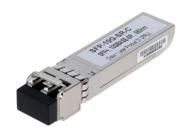
The enhanced small form-factor pluggable (SFP+) is an enhanced version of the SFP that supports data rates up to 10 Gbit/s. The SFP+ specification was first published on May 9, 2006, and version 4.1 published on July 6, 2009. SFP+ supports 8 Gbit/s Fibre Channel, 10 Gigabit Ethernet and Optical Transport Network standard OTU2. It is a popular industry format supported by many network component vendors.
